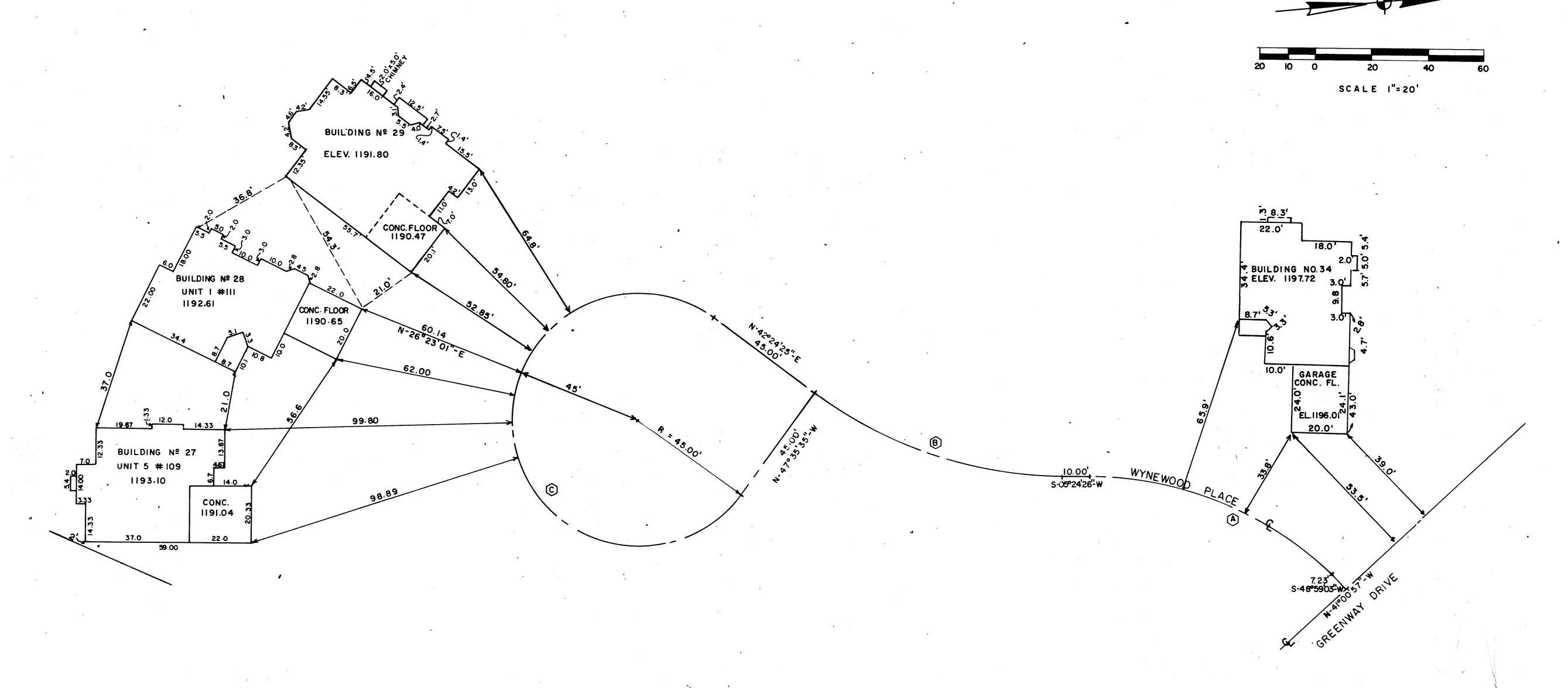
SITE AND LOCATION PLANS FOR THIRD (3rd) PHASE DEVELOPMENT OF BURLINGTON GREEN CONDOMINIUM. THESE PLANS SHOW THE FIRST FLOOR OF THE CONDO STRUCTURE CONTAINING BUILDINGS NO 27 THRU NO. 29 AND NO. 34, SEE SHEET 2 OF 3 FOR TOTAL PROPERTY CONFIGURATION.
